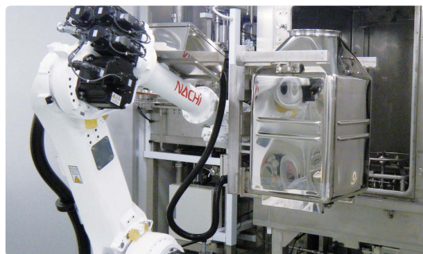
From insertion into the washer, container rotation, and transfer into the dryer, the whole process is done by robots
