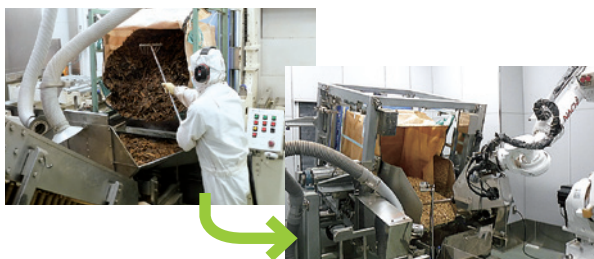
The Ibaraki Plant's third SD building, completed in December 2019, is fully automated. Realization of labor saving and robotization for the work of scraping crude drugs.
