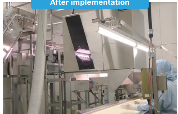
Crude drug sorting process conducted by a crude drug AI automated sorting machine and two persons
