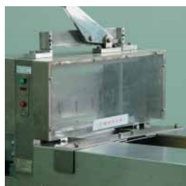
▲ Installation of safety cover of cutting machine
