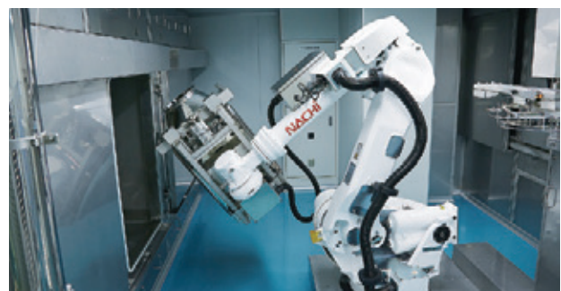
Lower : Robot arm to invert mixing containers
